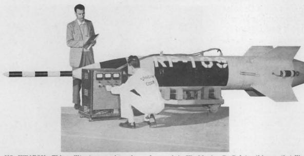
NO WEAPON—This militant appearing piece of hardware is a test vehicle used in Parachute study. Ben C. Benjamin, Supervisor of Sandia Corporation's Optical Measurements Division (5216) will speak in Washington D. C. later this month telling of Sandia's use of the cameras mounted between the tail fins, Left is G. Q. Wilson (5252) project engineer, and on the right is W. R. Drake (5212).
